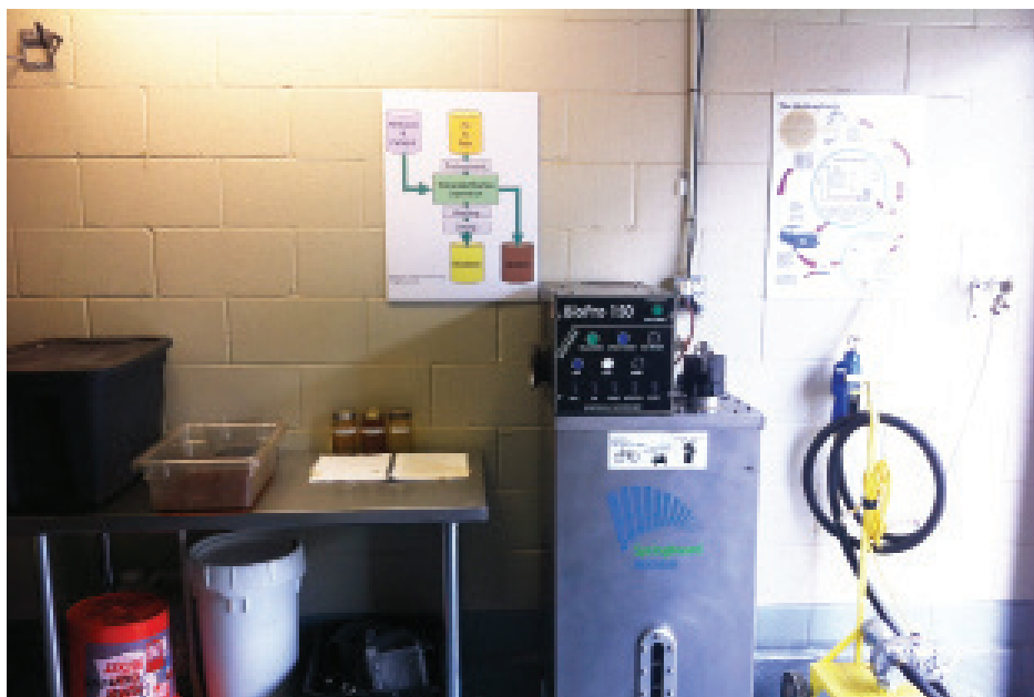
The BioPro 150 biodiesel processor turns waste cooking oil into fuel for the maintenance equipment at Tierra Verde Golf Club in Arlington, Texas. Photo courtesy of Mark Claburn
